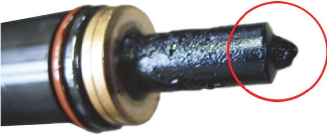
Fig. 3: Unit-injector element coked
