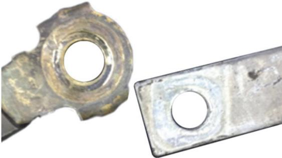
Fig. 1: Ground connection prior to cleaning: Poor connection
