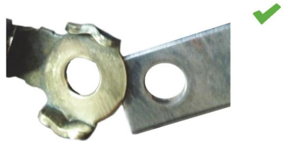
Fig. 2: Ground connection following cleaning: Good connection
