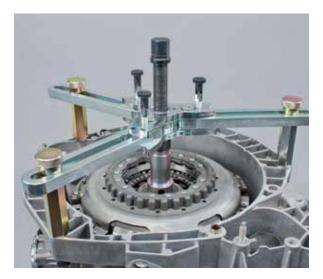
• Tighten the 3 Allen screws on the cross brace
