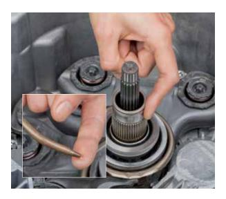
• Prepare the clutch for installation (mount the special tool)
