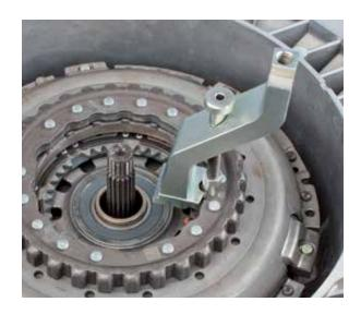
• Push the hook down and swivel into the clutch housing
