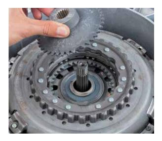
• Remove the retaining ring from the hollow shaft with the retaining ring pliers (KL-0192-12); the ring usually gets damaged in the process and needs replacing
