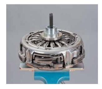
• At first, only turn the locking nut on the spindle far enough so that it rests against the adapter
