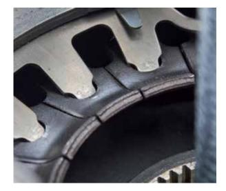
• Place thrust ring K1, Ø 85 mm (KL-0500-7110), on top of plate spring K1
