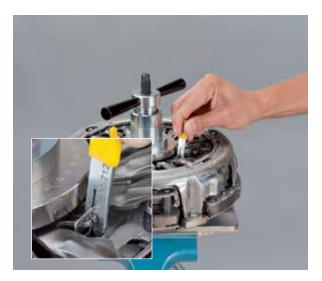
• Release the locking nut and unscrew (the locating lugs will fall over)
