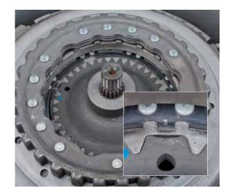
• Install the retaining ring in such a way that the abutting surface of the ring is centred on the metal tab, i.e. sits opposite the large tooth
