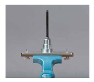
• Place the double clutch on the base plate with the plate springs facing upwards
