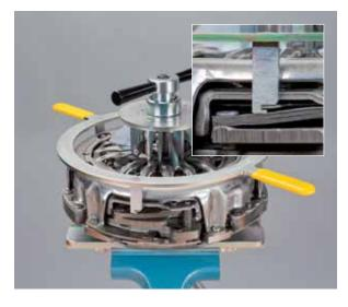
• Rotate the locating ring in an anti-clockwise direction (the direction of the arrow on the ring) as far as it will go and hold
