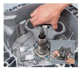
• Insert new lever actuators for K1 (wide fork opening). The correct position is determined by the guide sleeve and guide pin
