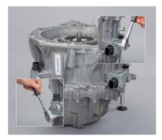
• Insert the release tool (KL-0500-8011) into the lever actuator for K2 with the marking (on the grooved surface) upwards
