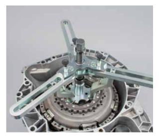
• Screw the knurled screw hand tight into the hooks
