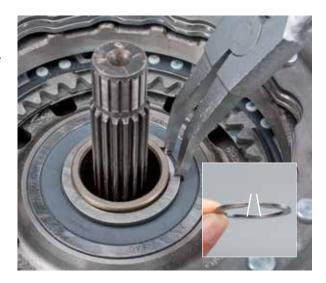
• Fit the clutch disc hub of the upper clutch disc (K1); installation is only possible in one position
