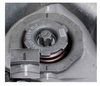
• Remove the transport lock from both lever actuators
