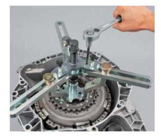
• Remove the clutch assembly from the hollow shaft by turning the spindle
