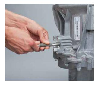
• Insert the release tool into the lever actuator for K1 with the marking upwards
