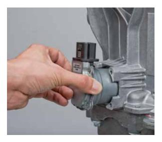
• Tighten the new screws on the base plate of the lever actuators to 19 Nm
