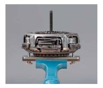
• Slide the locating pins into the teeth of the DMF attachment and tighten the knurled nuts
