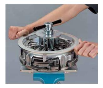
• Hold the locating ring in this position with one hand and screw down the locking nut with the other until the force needed to do so increases noticeably
