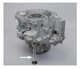
• Remove the retaining ring from the upper clutch disc hub (K1) using a screwdriver
