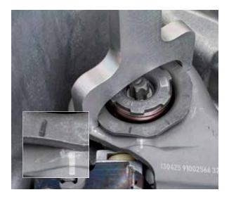
• Use the special open-end spanner (KL-0500-8010) on the housing of the return spring and turn it so that the markings are aligned facing each other
