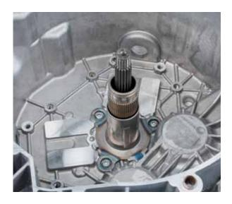
• Insert new lever actuators for K2 (narrow fork opening). The correct position is determined by the guide sleeve and guide pin
