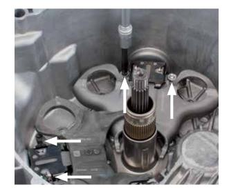
• Return spring and lever actuator are matched to each other at the factory and must therefore be correctly paired up
