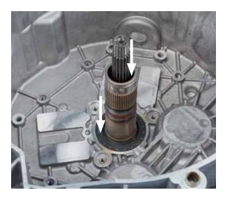
• Check that guide sleeves and pins are firmly seated
