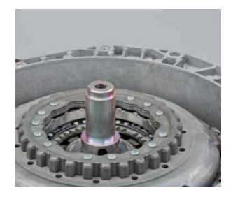
• Fit 3 threaded bolts (KL-0500-6021 or KL-0500-6022) to the gearbox housing using collar nuts
