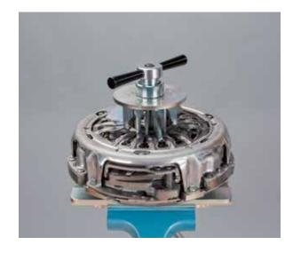
• Place the large locating ring for K2 (KL-0500-714) on the double clutch and fit into the tabs of the adjusting ring
