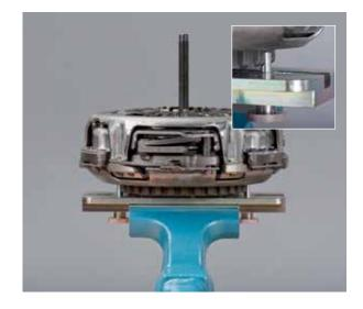
• Attach thrust piece K2, Ø 115 mm (KL-0500-716)
