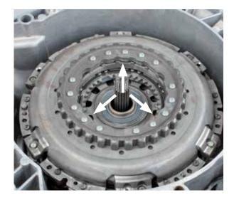
• Set the magnetic lifter of the hook on the clutch
