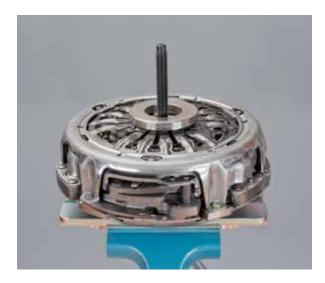
• Plug the adapter into the thrust plate
