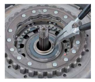
• Insert 3 hooks (KL-0500-824) each offset by 120° into the clutch assembly
