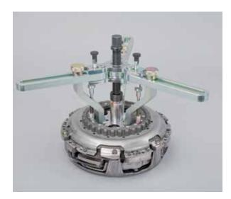
• Put the new clutch assembly on the hollow shaft; turning slightly ensures that the gear teeth of clutch plate K2 and the hollow shaft mesh with each other
