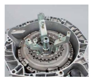
• Guide the locking piece (KL-0500-8210) with the central hole over the support sleeve and attach the hooks
