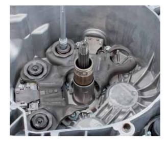
• Unscrew and remove the retaining bolts securing the lever actuators
