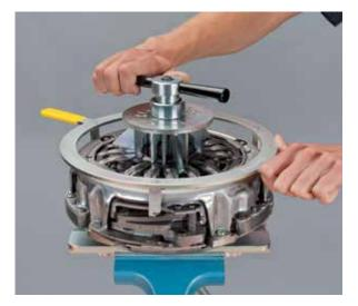
• Remove the clamping nut, locating ring claw fastener and locating ring
