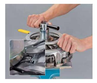
• Insert the tabs of transport lock K1 with the help of the locating lugs
