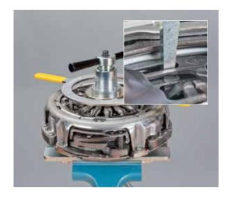
• Turn the locating ring in a clockwise direction (direction of arrow) as far as it will go
