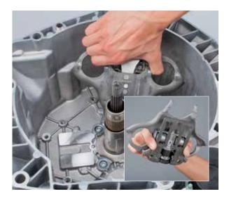
• Remove the 3 screws holding the centring sleeve
