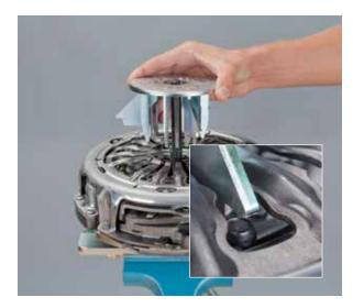
• At first, only turn the clamping nut on the spindle far enough so that it lies against the thrust piece
