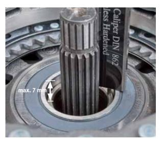
• Place thrust sleeve (KL-0500-8211) onto the bearing inner ring of the clutch assembly
