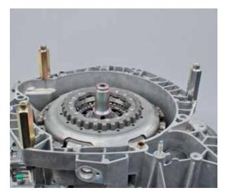
• Fix cross brace (KL-0500-60) to the threaded bolts using knurled screws (KL-0500-6020), ensuring that it is not under strain
